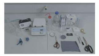
For the test, the textiles are cut into round pieces and stirred by magnetic mixers in a glass of liquid. After this process, the fibers are filtered and visually assessed. © Hohenstein
