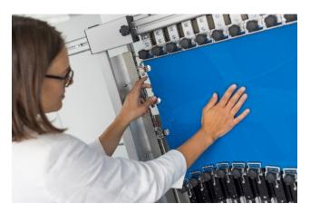
The Hohenstein HOSYcan testing device can be used to determine the compression effect of textile materials.
