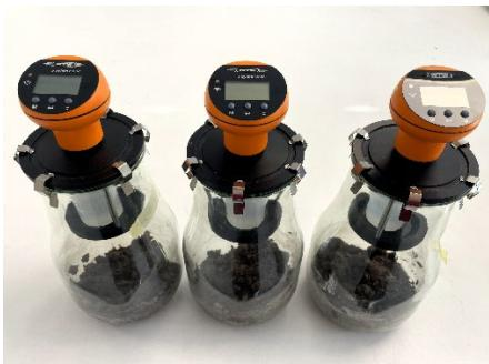
The respirometer system measures how much oxygen soil microorganisms consume during material degradation, determining the rate and extent of biological breakdown.
