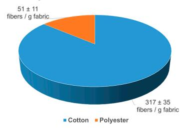
**Figure 7.** Fiber counts per g fabric of polyester and cotton fibers regarding the total amount of shedded fibers. These results refer to a wastewater sample from a washing process of a 50/50 polyester-cotton intimate blended fabric analyzed by dynamic image analysis.
