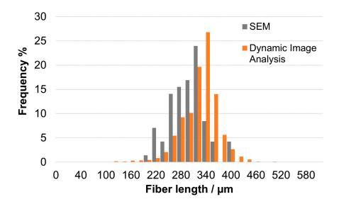
**Figure 3.** Distribution of the fiber length (0.3 mm polyamide 6.6 reference fibers) determined by scanning electron microscopy (SEM, grey columns) and dynamic image analysis (orange columns). A total number of 70 fibers was analyzed by SEM-imaging whilst > 5000 fibers were detected by a single dynamic image analysis measurement.
