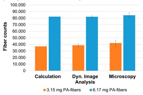
**Figure 5.** Results of the quantitative fiber determination of suspended polyamide 6.6 (PA-) fibers (0.3 mm length, 1.7 dtex). The fiber counts were determined for 3.15 and 6.17 mg fiber suspensions
