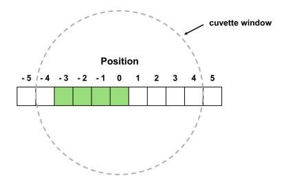
**Figure 2.** Cross-section of the dynamic image analysis flow-through cuvette. The horizontal axis is divided into  $3.75 \text{ mm} \times 3.75 \text{ mm}$  frames corresponding to the detection window. Positions 0 to -3 (green boxes) represent the experimentally accessible areas, whereas the remaining frames are not usable due to setup limitations.
