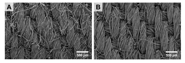
**Figure 6.** SEM-images of a 50/50 polyester-cotton intimate blended fabric. **A** Surface of the untreated fabric **B** Fabric surface after treatment with concentrated sulphuric acid. It shows a more aligned structure and a smoother surface after sulphuric acid incubation, confirming the removal of cotton.
