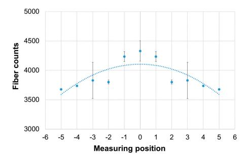
**Figure 4.** Fiber numbers determined by dynamic image analysis in correlation to the measuring position of the cuvette on horizontal axis. Fiber counts of position –4 and –5 are calculated values. A symmetric fiber distribution was assumed, and a quadratic curve fitting was applied.
